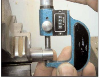
Figure 17. Measuring the shaft end.
