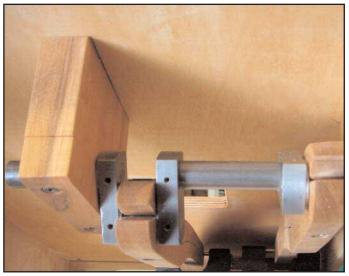
Figure 26. The crankshaft installed in an organ.
