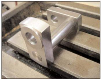
Figure 18. First two throws pressed onto the center shaft piece.
