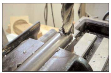
Figure 22 (above). Machining tapered square on the shaft end.
