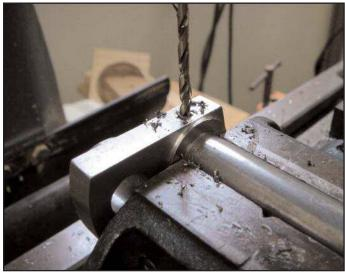
Figure 20. Drilling for a tension pin.
