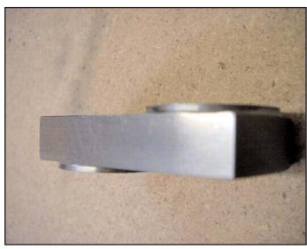
Figure 14. The completed crankshaft throw.
