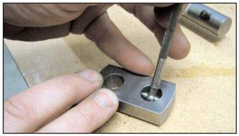
Figure 15 (above). Measuring inside diameter of throw.
