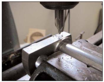
Figure 19. Center drilling for the tension pin.
