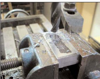
Figure 6. Drilling the crank throw.
