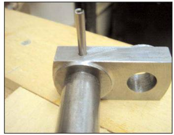
Figure 21. Installing the tension pin.
