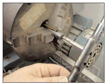
Figure 24. Tapping the shaft end.
