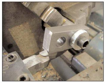
Figure 10. Machining the end of the throw.
