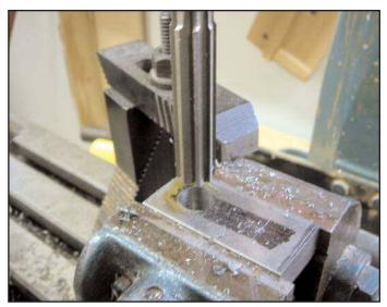
Figure 7. Reaming the drilled hole.
