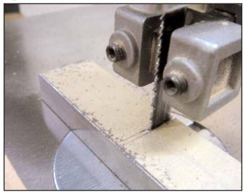
Figure 3. Stock marked to allow for removal of saw cut.
