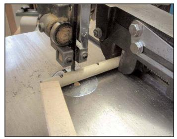
Figure 2. Cutting shaft stock with a band saw.
